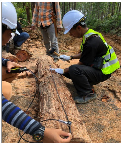
Figure 3. Assessment of acoustic velocity on billets of E.pellita
