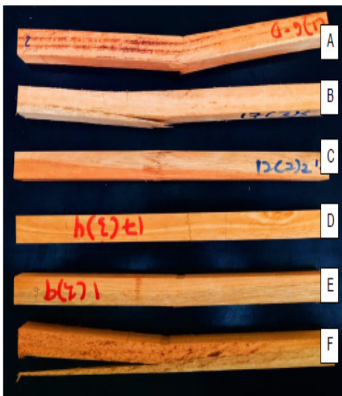
Figure 10. Types of failure mode in bending test
