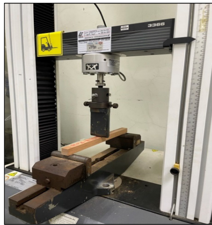
Figure 5. Set up for the 3-point flexure bending test
